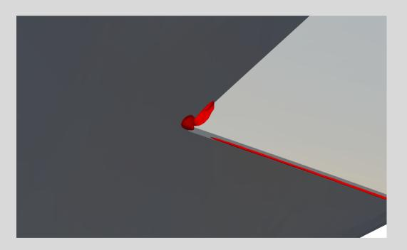
Showing Iso-contour of Ux=-10. Wing-body separation as expected.
