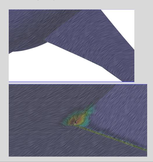
Rest of the plane is clean with the only expected separation in the junction region
