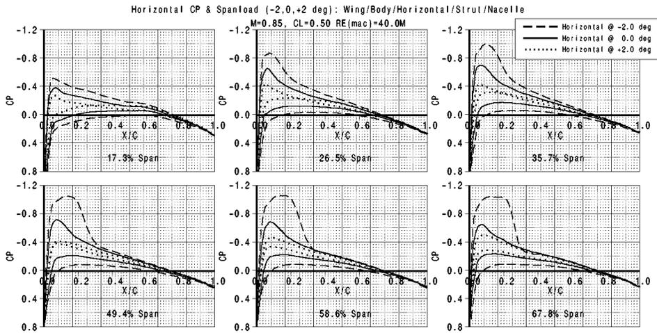
Figure 19: TRANAIR Results of CRM Horizontal-Tail Pressures.
