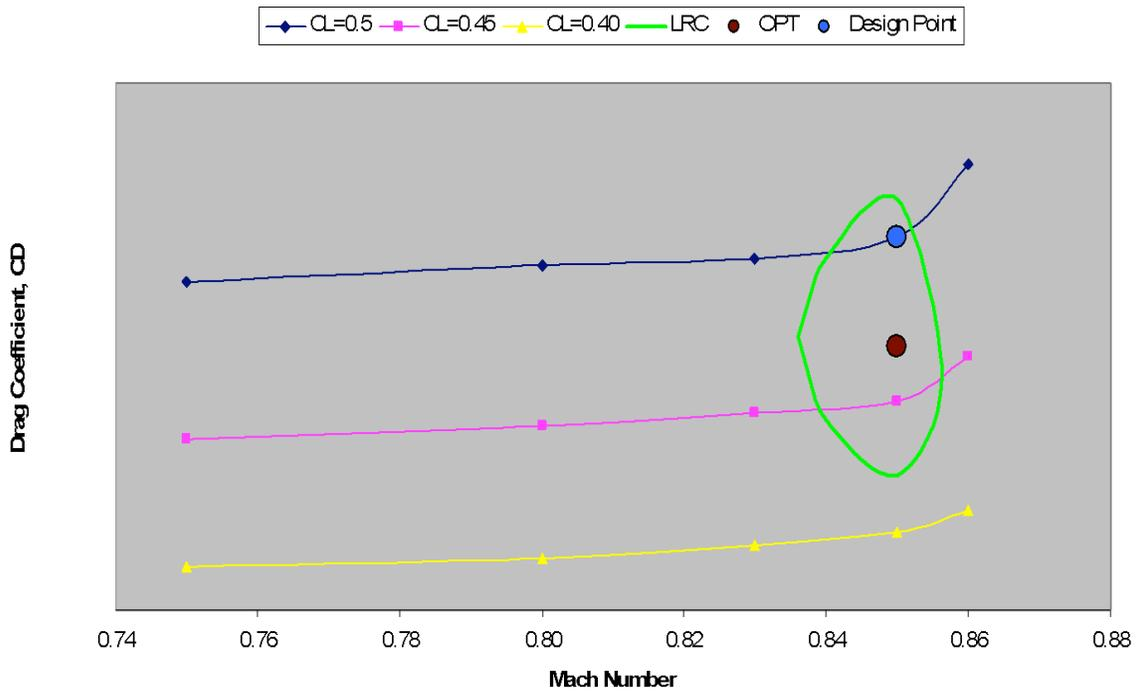
Figure 15: OVERFLOW Drag Rises for the CRM Wing/Body.
