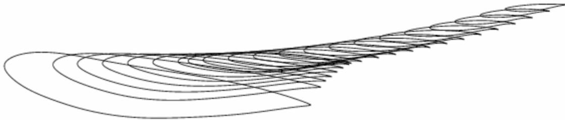
Figure 2: Airfoil Stack for the CRM Wing.
